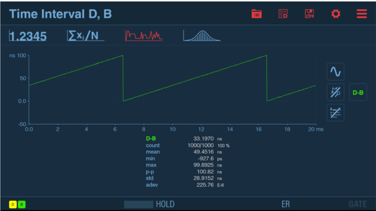
Fig. 5.6: Time Interval Continuous of 2 clock signals with constant frequency offset
