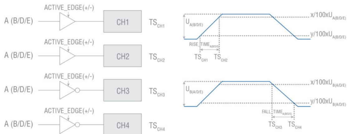
Fig. 5.17: Rise Time and Fall Time measurement
