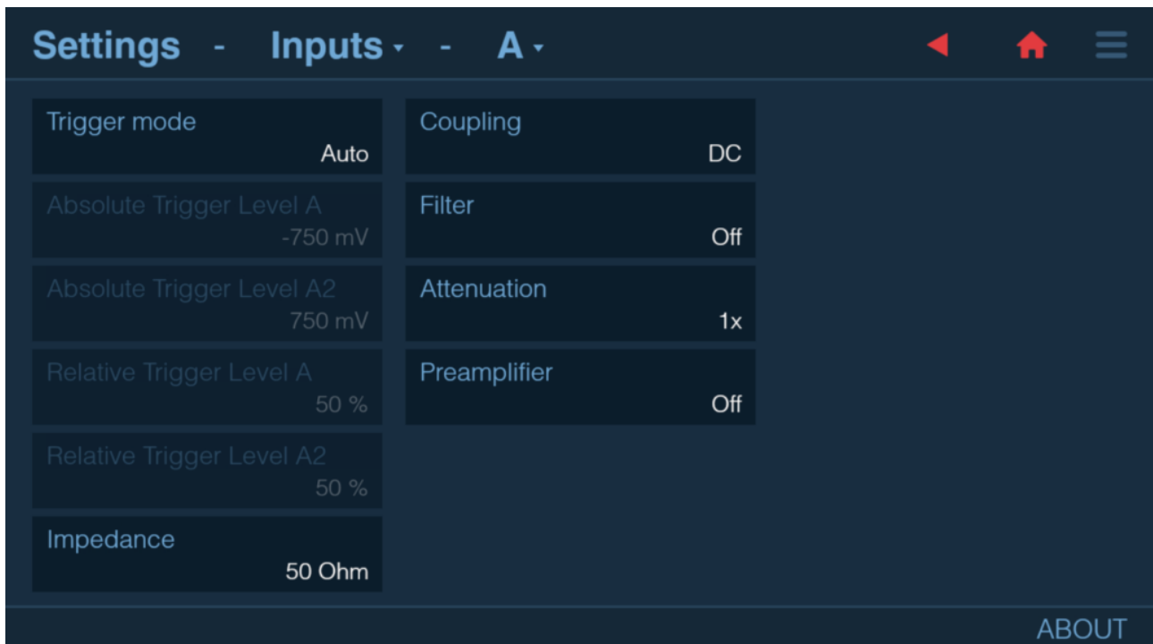
Fig. 4.6: Input amplifiers configuration menu
