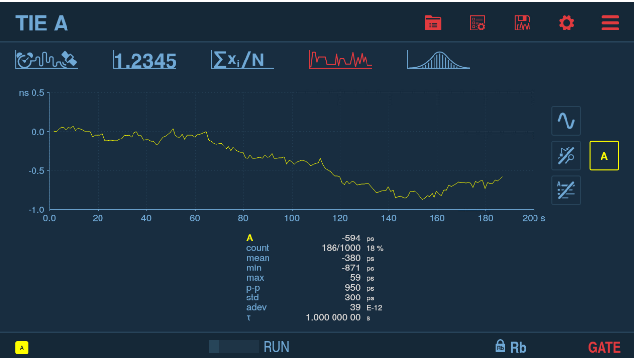
Fig. 4.6: Example of TIE measurement trend graph
