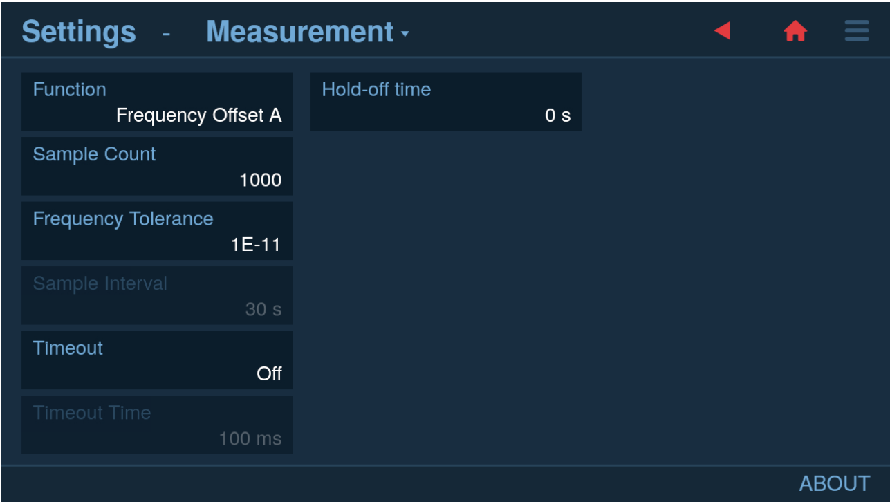
Fig. 4.4: Setting calibration tolerance for Frequency Offset function (Frequency Tolerance setting)
