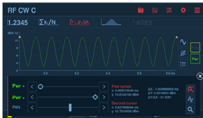
View fast FM/AM, or any time/phase/frequency/power modulation, on screen. This example shows AM with 10 kHz modulation. Modulation period (100 \mu s) is measured via cursor read-out over 10 modulation cycles.
