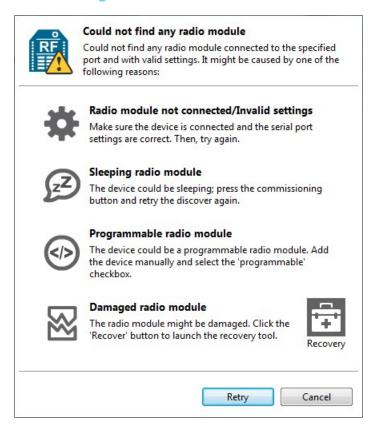
**Note** You can also use the Add a radio module dialog to add programmable radio modules. See Add a programmable radio module.
