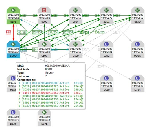
■ Each node is connected to its neighbors with solid lines (active connections) or dotted lines (undiscovered connections), with arrows indicating the direction of communication. Selected nodes are blue, and connections are black. Nodes discovered in previous scans that have not been found in
