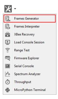
**Note** You can also access the Frames generator tool from the API console when you add a new API frame to the list of frames to send. Use the **OK** button to automatically copy the generated byte array to the content of the frame to be added.
