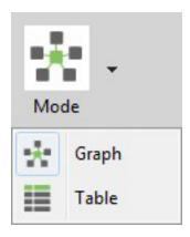
In Graph view, XCTU displays the modules as nodes in a graph. A green background denotes the local radio module and a blue background denotes the selected module. Each module is labeled with its role (coordinator, router, or end device) and MAC address as well as the 16-bit network address for ZigBee networks and node identifier for other protocols. You can click any node to inspect its connections.
