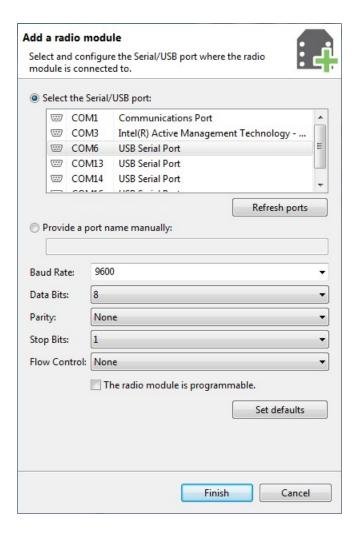
2. Select the serial port where the radio module is connected (or enter its name manually) and configure the serial settings of the port.
