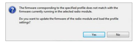
If the firmware of the configuration profile is not compatible with the radio module, click
