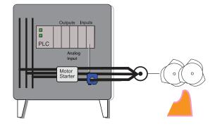
Monitor a shredding operation to measure current usage, enabling automatic shut down if the blades become jammed or overloaded.
