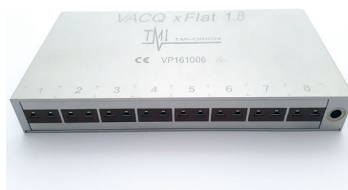
VACQ xFlat 1.8 with connectors for type T thermocouples
