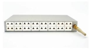
VACQ xFlat 2.8 universal FullRadio, with 16 miniature connectors for thermocouples
