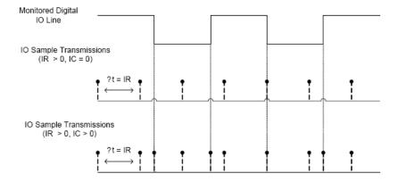
Enabling Edge Detection will force an immediate sample of all monitored digital IO lines if any digital IO lines change state.
