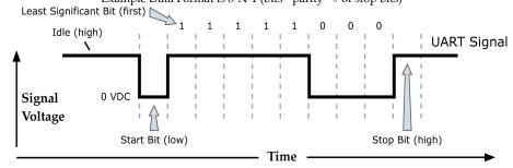
The module UART performs tasks, such as timing and parity checking, that are needed for data communications. Serial communications depend on the two UARTs to be configured with compatible settings (baud rate, parity, start bits, stop bits, data bits).
