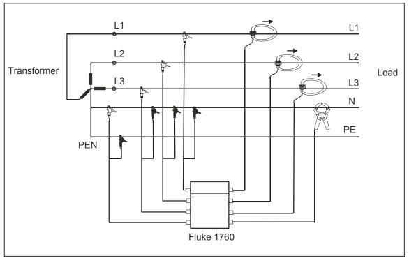
Figure 3-5. Circuit Diagram: 4-Wire
