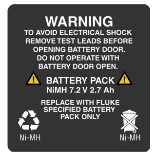
Figure 1-2. Instrument Labels
