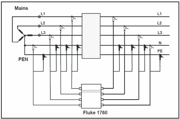
Figure 3-6. Circuit Diagram: 2 Voltage System with Neutral
