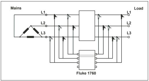
Figure 3-7. Circuit Diagram: 2 Voltage System in Delta Connection
