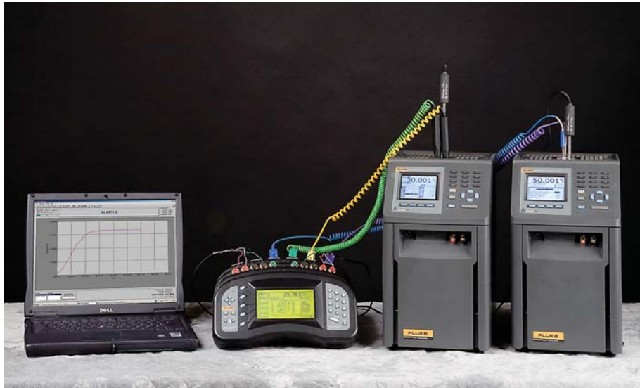
The Black Stack is the perfect foundation to build a totally automated calibration system with Hart heat sources and 9938 MET/TEMP II software (see page 97). No programming or system design nightmares.
