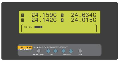
Figure 46 Select Calibration Channel
