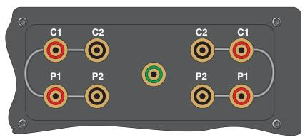
Figure 49 Using a Shorting Wire
