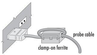
Figure 1 Using the Clamp-on Ferrites
