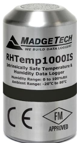
The new RHTemp1000IS is MadgeTech's most robust temperature and humidity data logging solution. FM Approved to be Intrinsically Safe for Class 1, Division 1, groups A, B, C, and D and non-incendive for Class 1, Division 2, groups A, B, C, and D, the RHTemp1000IS is certified as safe for use in many hazardous locations where explosive gas atmospheres are present.
