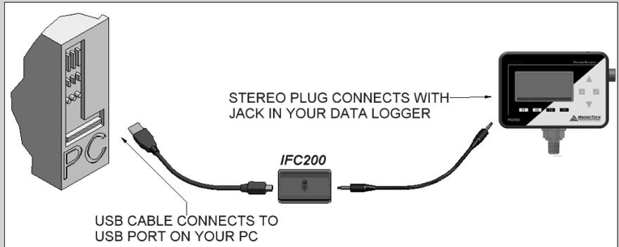
Insert the USB connector of the IFC200 into an available USB port. Fully insert male connector of the IFC200 interface cable into the female receptacle of the data logger\*.
