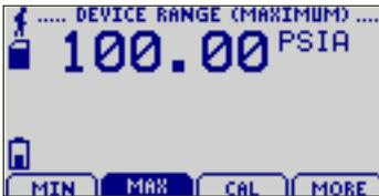
*Displays values indicating maximum pressure detectable by the PR2000.*
