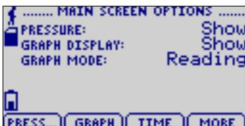
*Displays options for changing the view on the main screen (either shows a particular channel or hides it).*
