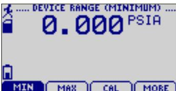
*Displays values indicating minimum pressure detectable by the PR2000.*
