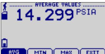
*Displays statistics from from the pressure channel sorted by type (maximum recorded value, minimum recorded value, or average value).*
