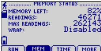
*Displays information about the device's memory capabilities including percent of memory available (memory left), number of readings taken so far (readings), max number of readings (max readings), and wrap status.*
