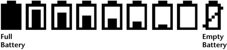
Battery status icons indicate the state of charge of the batteries. When the battery empty indicator is displayed, the battery should be replaced.
