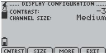
*Allows the user to change the contrast of the LCD display as well as the channel size.*
