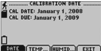
*Displays date of last calibration and due date of next calibration.*
