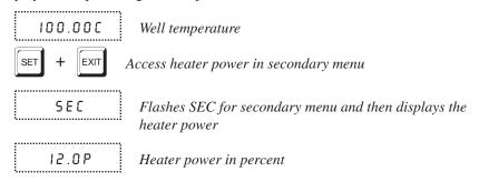
To exit out of the secondary menu press "EXIT". To continue on to the proportional band setting function press "SET".
