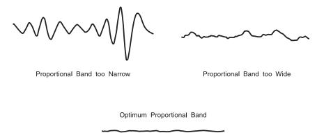
Figure 5 Temperature fluctuations at various proportional band settings
