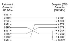
Figure 6 Serial Cable Wiring
