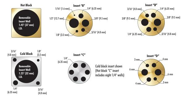
Figure 3 Interchangeable Insert Options
