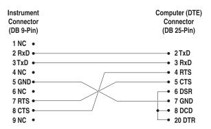
Figure 9 Serial Communications Cable Wiring
