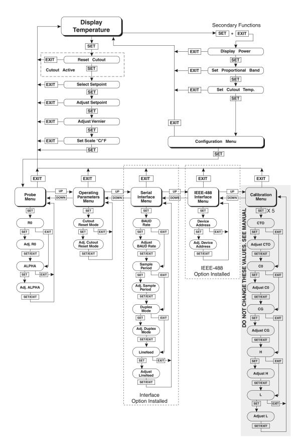
Figure 7 Controller Operation Flowchart
