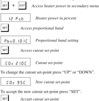
The next function is the configuration menu. Press "EXIT" to resume displaying the bath temperature.
