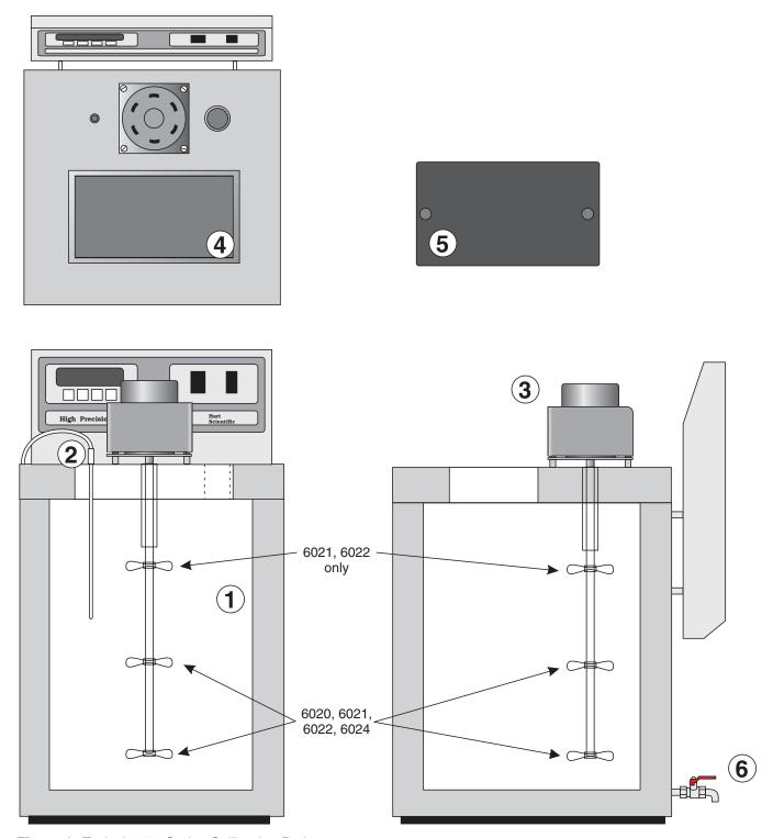
Figure 4 Typical 6020 Series Calibration Bath
