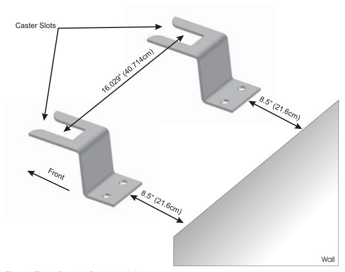
Figure 2 Tipping Prevention Bracket Installation
