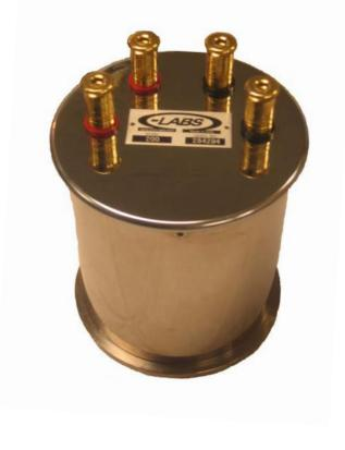
In addition to decade values, the 200-Series are offered in –T values for thermometry, and –Q values for use with a Quantum Hall System.
