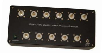
Guarded high resistance transfer standards allow accurate 100:1 build-up of high resistance.
