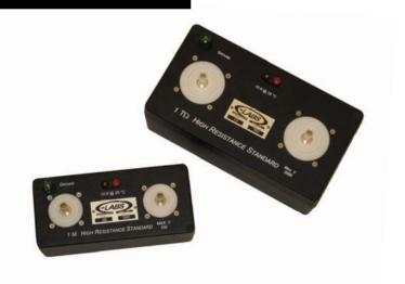
The guards are internally connected by a high value resistor, to provide a guard current path.
