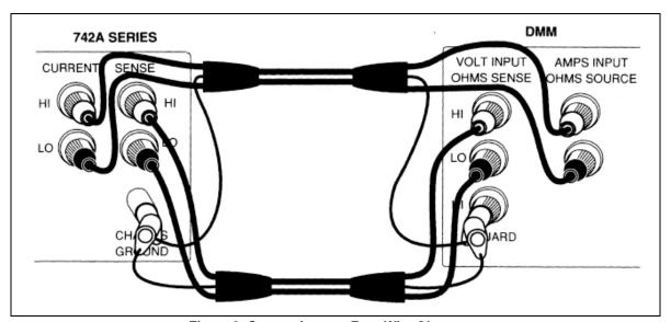
Figure 3. Connection to a Four-Wire Ohmmeter
