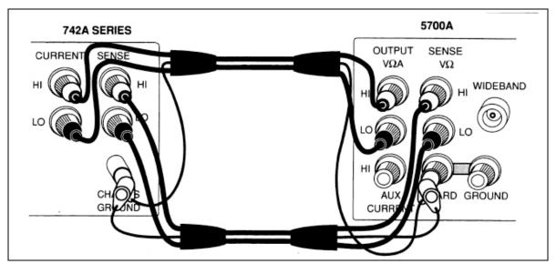
Figure 4. Connection to Calibrate the 5700A
