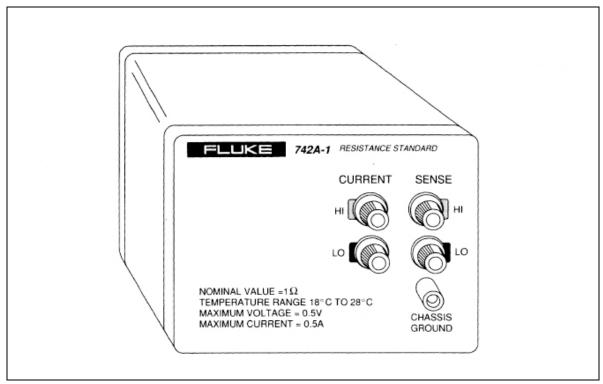
**Figure 1. Typical Front Panel View**
