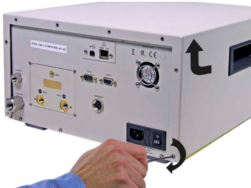
Figure 29. Removing Back Cover
