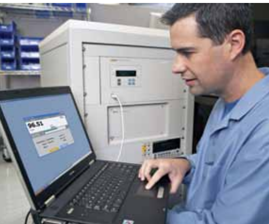
PPC4 standard front panel USB connection provides easy access and use of "cockpit" software for full PC based plug-and-play functionality
