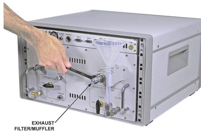
Figure 5. Installing the exhaust filter/muffler
