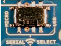
With the switch in the **USB** position, the DOUT pin the wireless module is connected to the RX pin of the USB-to-serial converter, and DIN on the wireless module is connected to the TX pin of the USB-to-serial converter. This means that the module can communicate directly with the computer. The microcontroller on the board will be bypassed. **To use the shield in this mode**, **you must program the microcontroller with an empty sketch (shown below)**, **or remove it from the board**.
