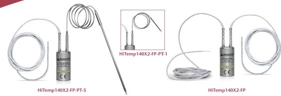
The HiTemp140X2-FP series of dual probe high temperature data loggers are comprised of a stainless steel data logger body and feature two 36 inch or 72 inch flexible FP probes or are available with one flexible probe and a stainless steel bendable PT probe combination.
