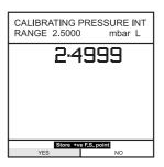
After application of the final calibration pressure, the calibration results are displayed as shown below. To view the second page of calibration data press MORE (F1). Press ENTER complete the pressure calibration procedure.
