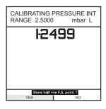
Apply the fifth and final calibration pressure( positive full scale) and store the positive FS point as shown below (e.g.),
