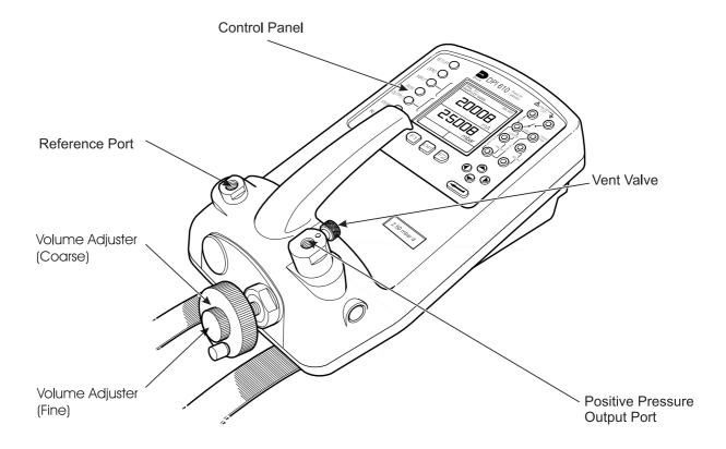
Figure B1 - DPI 610LP Calibrator Controls
