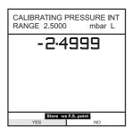
Apply second calibration pressure(negative half full scale) pressure and store the half -ve FS point as shown below (e.g.),
