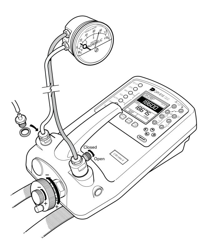
Figure B2 - DPI 610LP Test Connections
