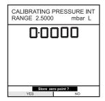
Apply fourth calibration pressure (positive half full scale) and store the half FS point as shown below (e.g.),
