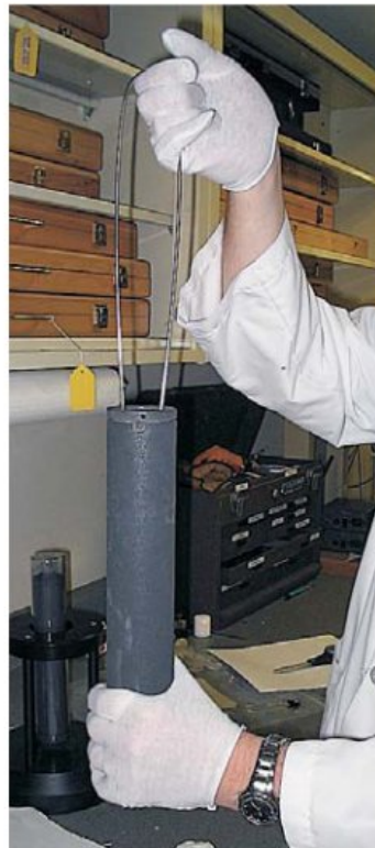
Figure 24 Preparing basket assembly for installation in furnace.
