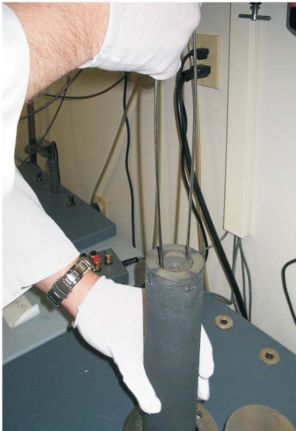
Figure 25 Installing basket assembly in furnace.
