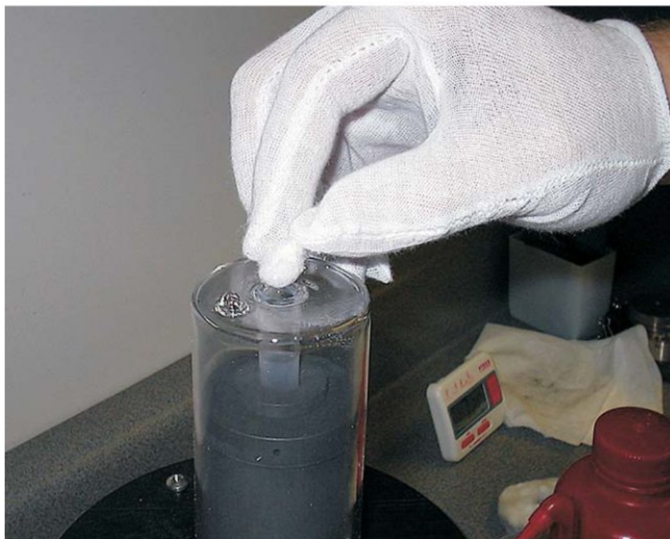
Figure 13 Place insulation in re-entrant well.
