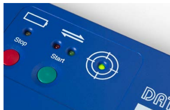
ET3 logger SmartPaq* – “Pass/Fail” indication from logger
