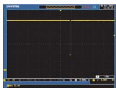
SEQ6: Momentary Drop in Supply Voltage
