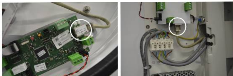
RJ45 Ethernet port: Single-sided (left) and Double-sided (right)
