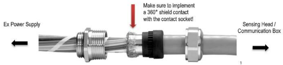
Figure 45: EMC Compliant Connection for the Cables for Sensing Heads and Communication Box
