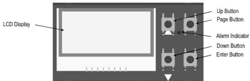
Figure 33: Control Panel for the Comm Box (DIN)
